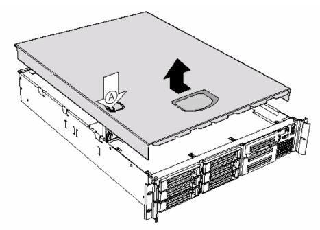
Figure 8: Removing the Cover
